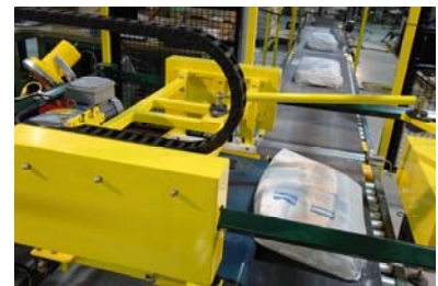
Bag conveying system incorporating belt over roller
