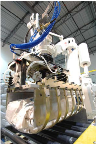
KRAKEN engineered robotic end-of-arm tool for squaring, gripping and placing product
