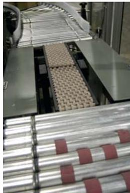
control. No other mechanical setup or adjustments are required. This functionality provides operators with optimum, uninterrupted flow and control of cases being conveyed. Moreover, systems can be configured for conveying and orientation on more than two (2) axes, and can be adapted to perform random orientation by scanning bar code SKUS on cases.
